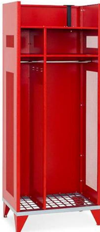
The special cupboards for fire and rescue services are an assembled construction made of 1 and 1.3 mm thick sheet steel. The cabinet is open so that clothing and equipment can be accessed immediately during an operation. The side walls are perforated so that the clothing can air out sufficiently. The steel shelves can be equipped with feet (height 100 mm) and levelling screws. With the special tiltable helmet holder it is possible to remove the helmet more easily.
