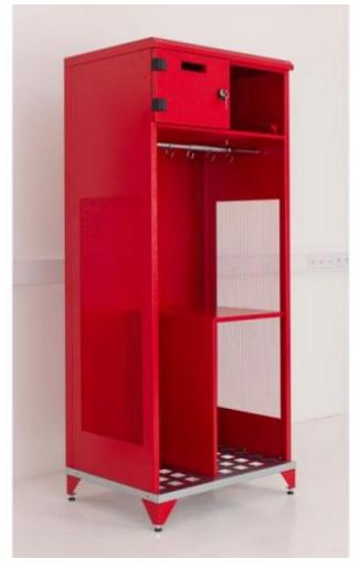
It is a welded construction made of 1 mm thick sheet steel. They guarantee the immediate availability of emergency clothing whenever it is needed. The steel grids can be fitted with adjustable feet (height 100 mm). For an extra charge, the lockers can be equipped with a special flip-up helmet holder. By simply pulling on the helmet, the holder folds down, making it much easier to remove the helmet.
