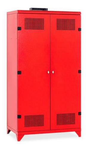
The special cupboards for fire brigade and rescue units are a welded sheet steel construction made of 1 mm thick sheet metal, these fire brigade cupboard systems can be equipped with a dryer for an extra charge. The door is closed by a rotary bolt which allows quick access. The floor is perforated and extra reinforced. The cabinets have a special lockable compartment with a throw-in slot for small items.
