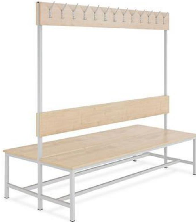
Cloakroom benches are used in changing rooms in companies, gyms, schools and sports clubs. They are made of robust 30 x 30 mm steel profiles. The seat surface has a laminate top with a 2 mm wide ABS edge. The feet are equipped with plastic glides and the backrests have practical hooks in the respective profile colour.
